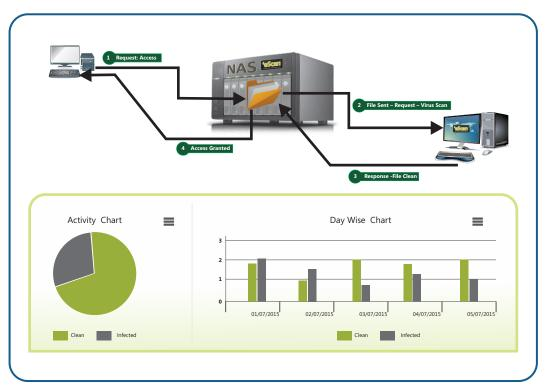
Files are saved on NAS Server, whenever a File Access request is received by the NAS Box, the file is sent to eScan for NAS for Virus scanning. After scanning if the File is found clean, access is granted to the user or denied in case the file is infected. Access Granted or Denied and conditions for the same are configured in Oracle ZFS storage appliance control panel. After receiving the results received from eScan for NAS, corresponding command is executed.
